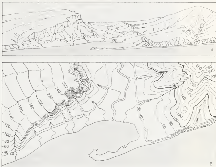
Figure 7: Landscape shown in perspective A is represented with the aid of contour lines on map B.
